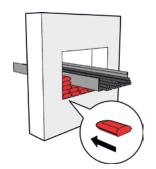
Insert the RPS-T Firestop pillows in the recess so that the long side of the RPS-T Firestop pillows is parallel to the conduit.
