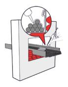
At the site where the RPS-T Firestop pillows are to be inserted, apply RPI-S Filler between the cables and in the profile of the conduit over a width of about 200 mm.
