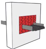
Fill the rest of the recess with RPS-T Firestop pillows until the whole recess is sealed. Here too, pack the RPS-T Firestop pillows in as tightly as possible so that no joints are formed.
