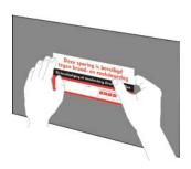
Fill in the working data on the RPI-S Seal sticker and attach it in clear sight.
