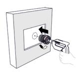
Set the drill in the right direction and place the saw up against the (mineral wool) board.
