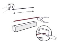
First measure the required length of the RPI-D Intumescent strip, Door strip or Smoke strip and adjust the length if necessary.
